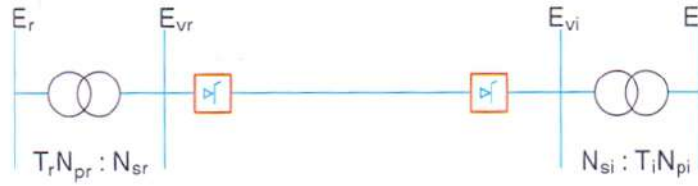
Fig. 4.1: (b) Schematic of a DC link showing transformer ratios
